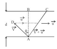
Swimmer heads along AD making angle  $\theta$  with vertical in the direction of upstream so as while it crosses the river it has less drift along the direction of river flow.
